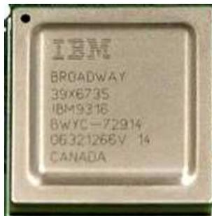
Figura 66 – Processador IBM Broadway.
